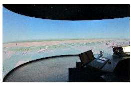
APP and 3D Tower Simulator in Casablanca, Morocco In 2010, the Mohammed VI Civil Aviation International Academy, chose Tern Systems to design, customize and deliver a 3D tower simulation solution for the academy. The facility consists of a 180° curved screen simulator with 2 controllers and
